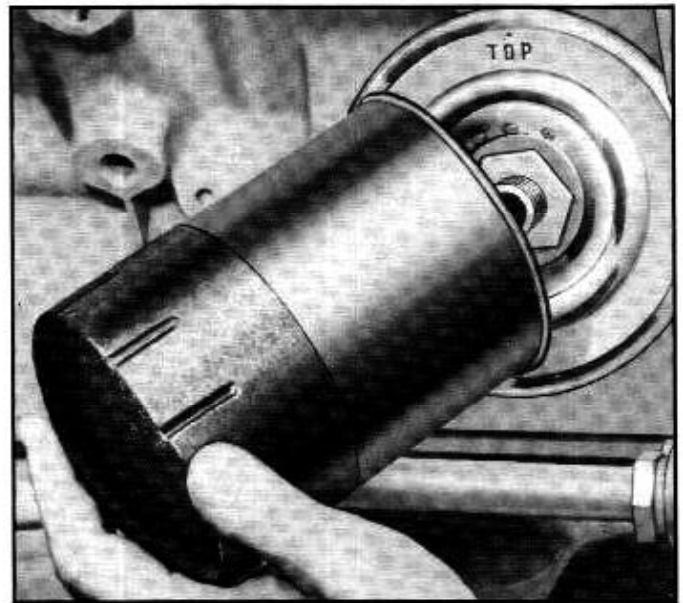
Fig. 6A-18—Oil Filter Replacement
