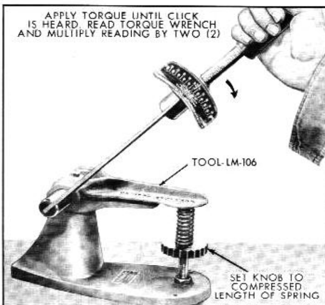
Fig. 6A-43—Testing Valve Spring Tension
