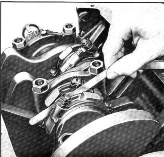
Fig. 6C-147—Checking Connecting Rod Side Clearance
