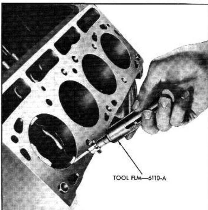
Fig. 6C-102—Checking Piston Clearance
